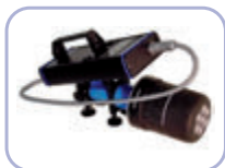
Step OD-02 misura dose e rateo H*(10) e H (0,07) 8 KeV - 15 Mev RX (nanopulstate), Gamma e beta
